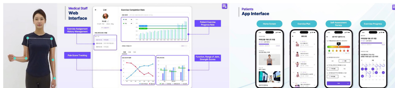
Fig. 2. A company utilizes machine learning-based pose estimation technology to measure a patient's range of motion, analyze the patient's current condition based on the results, and assign the most suitable rehabilitation exercises. This figure is used with permission from Itphy, Inc.
